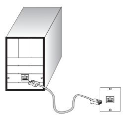
Figure 4-1 Making Twisted-Pair Connections
